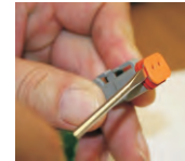
Remove the orange wedge by lift the wedge from the connector with a small flat head screw driver or Deutsch connector tool.
