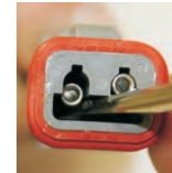
Extend the Actuator: White Terminal to Positive (+) Battery Terminal. Black Terminal to Negative (-) Battery Terminal.
